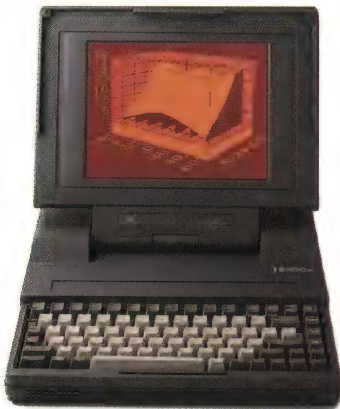
T3100e: 12MHz 80286, internal IBM slot, 20MB hard disk, gas plasma display, 1MB RAM expands to 5MB, 1.44MB 3 1/2" diskette drive.
